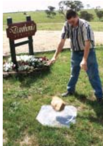
We tested several materials to protect the lead lighting, and broke at least one sample before finding the best product for the job. Here's our R&D specialist completing an impact test. The polycarbonate didn't break.
